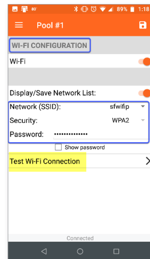
Fig. 10.17: Test Wi-Fi Connection
